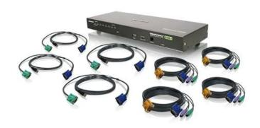
The GCS1808KIT KVM is a combo VGA switch that includes 8 KVM cables - Set of 4 USB and 4 PS/2 KVM cables.
