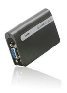
The USB 2.0 External VGA Video Card allows you to connect an extra monitor to your desktop PC or laptop's USB port. The connected monitor can be configured to either clone your primary screen, or extend the Windows desktop allowing visibility of more applications at the same time.
