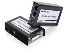
IOGEAR's DVI-D CAT5e/6 Extender with Stereo Audio gives you the distance between the 1080p (1920x1080) media source and the HD display unit by you're connecting by up to 130 feet. It consists of a local sending unit and remote receiving unit connected by two standard solid CAT5e/6 twisted pair solid Ethernet cables. Additionally, you can extend up to 200 feet\* at 720p resolution.
