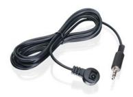
The GWIR8101 is an infrared (IR) extender for the GWAV8141K (Wireless Receiver) allowing you to hide the wireless receiver and still have wireless remote control over your home entertainment source devices. It is a 3 conductor connector with dual bandwidth (Dual Band) 38KHz and 56KHz support for all the latest devices.
