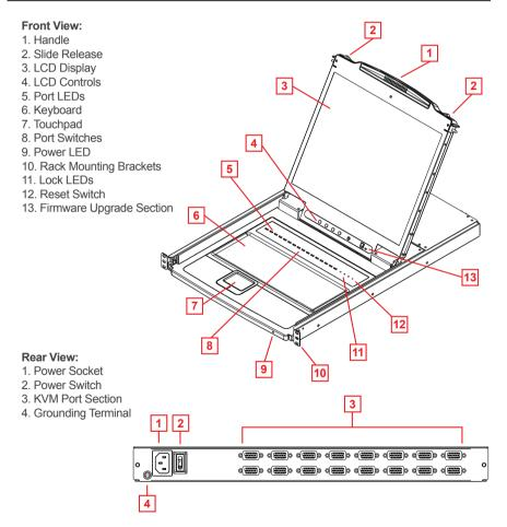
**Note:** The GCL1916 is pictured above. The GCL1908 rear panel is the same as the GCL1916, except that it has 8 KVM ports instead of 16.
