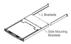
**Step 1**While one person positions the switch in the rack and holds it in place, the second person loosely screws the front brackets to the rack.
