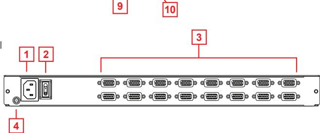
**Note:** The GCL1916 is pictured above. The GCL1908 rear panel is the same as the GCL1916, except that it has 8 KVM ports instead of 16.
