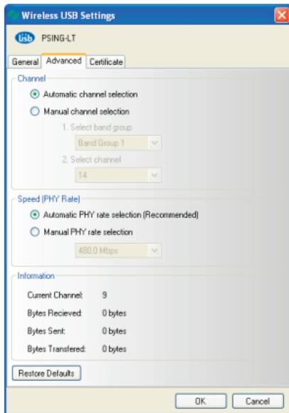
If required to change the Channel manually, select **Manual channel selection**. The following figure shows the available channels for selection.
