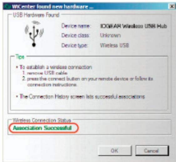
After completing the association process, unplug the USB A to mini B cable from the Wireless USB Hub.
