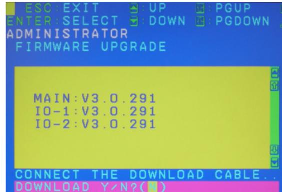
After you type Y, you will see the below screen. The KVM is now in firmware upgrade mode. Please see Firmware Upgrade section for details about how to perform a firmware upgrade.
