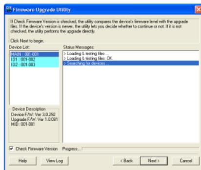
\*Note: Please choose MAIN to proceed the firmware upgrade. IO1 and IO2 are sub layers in the KVMs firmware.
