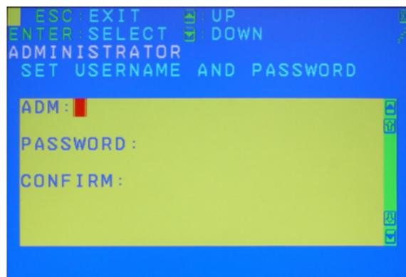
Once the user name and password are set correctly, you will see the message in the bottom of the screen indicating the setup is ok. Then simply press [Esc] to exit from the function.
