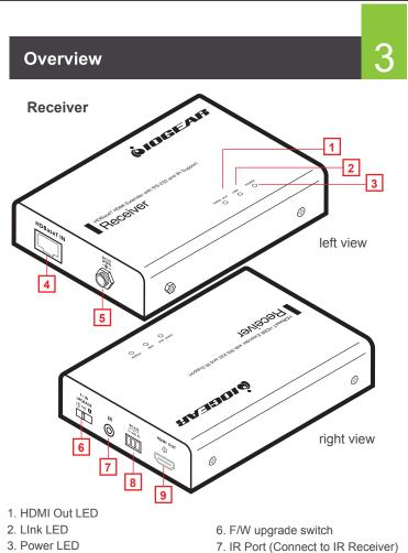
7. IR Port (Connect to IR Re 8. RS-232 Port 9. HDMI Output Port
